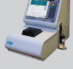
measure four specified properties at the same time-viscosity (at +40° C), density, cloud point, and pour point—in 20 minutes or less, which greatly improves productivity.
